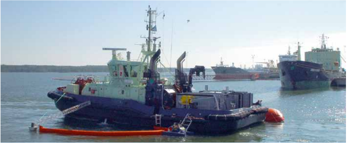
Neste Oil's Ahti escort tug can also be used in oil spill prevention and response work.
